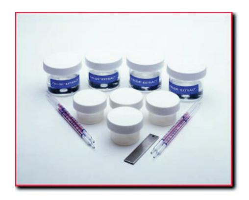
An easy to use, accurate field test for chloride contamination of abrasives
