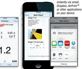
PosiTector SmartLink accepts PosiTector 6000, SPG, RTR-H, and DPM probes easily converting to a coating thickness gage, surface profile gage or dew point meter.
