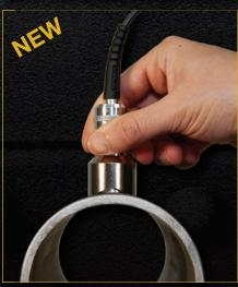
**NEW** surface profile probe for outside diameters
