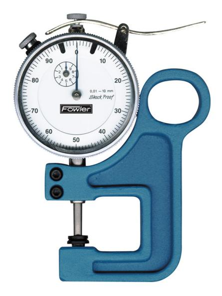
Fowler's Dial Thickness Gages are light in weight, easy to handle and carry. These specially built gages are mounted in a hand contoured frame with a thumb release mechanism; has fast direct reading to .001". Used to measure thickness of paper, cellophane, plastic film and metal plates. These are high quality precision instruments.
