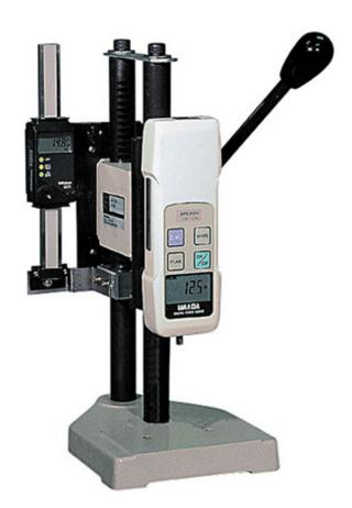
The NLV-220 lever operated force measurement test stand provides an affordable, reliable, and easy to use means of performing consistent force testing. The NLV-220 is Imada's most economical test stand. Compared to testing by hand, using a test stand will greatly increase the repeatability of any test.
