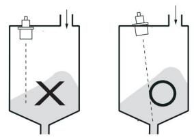
As is illustrated by the figure on the right, the transducer should be mounted on the top of guide tube to prevent the false echoes from turbulence and foam. The guide tube should come with a vent hole at top of the tube to allow the liquid vapor go out of the tube.
