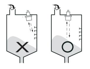
The transducer should not be mounted too close to the tank wall, the build-up on the tank wall cause false echoes.
