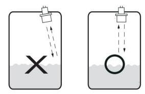
Mount the transducer away from the inlet to avoid false echoes.
