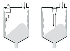
When you mount the transducer on the solid tank, the transducer must point to the tank outlet.
