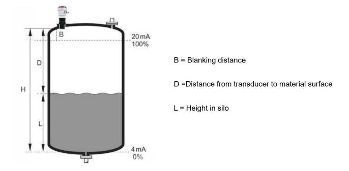
The distance D is determined from the velocity of sound and the time period t by the formula:
