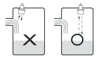
The transducer should not be mounted too close to the tank wall, the bracket can cause strong false echoes.
