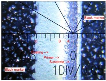
Line "A" mark s the edge between substrate and primer. Line "B" is the line between primer and top-coat. Line "C" is the top of the coating, made easier to see by using the black marker.
