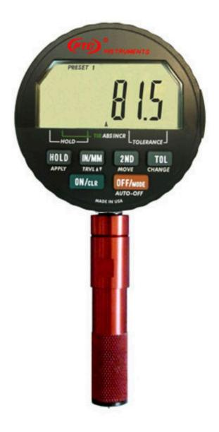
D Scale Durometers Measure the hardness of pipeline coatings, plexiglass, epoxy, vinyl, cellulose acetate, and other similar materials.
