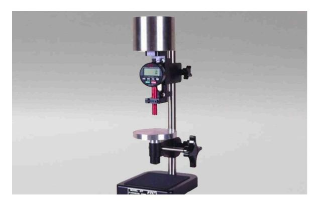
This stand is for use with PTC®'s line of pencil style durometers and is also fully compatible with durometers of other manufacture. The Model 477 has a 5 kg weight and is for use with ASTM Type C, D and DO pencil durometers.
