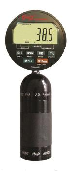
ASTM Type OO Durometers measure the indenter hardness of polyethylene foam roll, sponge rubber, very soft rubber.
