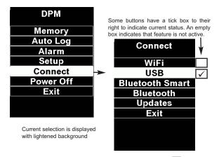
To navigate, use the Up and Down buttons to scroll vertically and w to SELECT.
