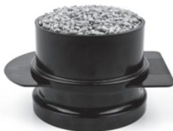
When these actions are completed, place the filled dispenser on the chamber (bottom edge of the dispenser is specially profiled to match the GMM mini casing). Then remove the damper to fill the measurement chamber with grain.
