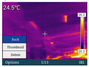
Press "+" or "-" to select "back", "thumbnail" and "delete" menu, and press "back" key to back to the main interface. If you select "thumbnail" and press "confirm" key to access "thumbnail" menu, under this menu, press "+", "-", " ◄" and "▶" to select corresponding images with such keys and conduct deletion, full-screen preview and other operations of such images, as shown below.
