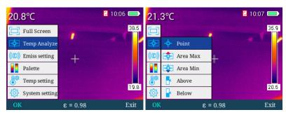
Test temperature of central point in "point" analysis mode, as shown below.
