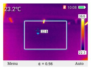
In "upper isotherm" mode, select high-temperature color band with "+" and "-" keys and display it in red. Meanwhile, display corresponding high temperature area in real-time image, as shown below.
