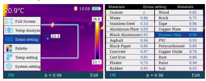
It is also allowed for user-defined emissivity value. In emissivity mode, go to custom mode, select "confirm" key, and then press "+" and "-" keys to customize emissivity value ranging from 0.01 to 1.00. Press "exit" key to back to main menu.
