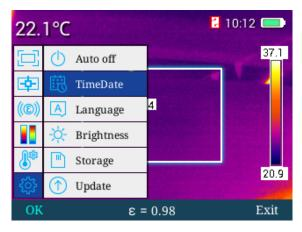
In "time and date" menu, press "▶" to successively select values to be adjusted which will be highlighted in blue, and then select "+" or "-" keys to adjust values selected. Press "◄" key to back to previous value selected and press "confirm" key to save current value adjusted, as shown below.
