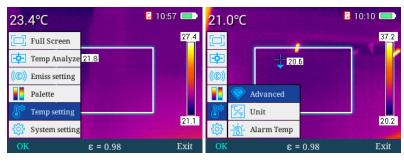
Then press "confirm" key or " > " key to go to "advanced" menu where you can adjust numerical values of reflected temperature, relative humidity and temperature measurement distance, as shown below.
