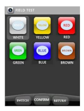
Place the front of the detector against the tested material. Make sure the light could not enter into the tested area. Pull the trigger to start testing, 5 seconds (2 seconds if continuous measurement) later the result will be shown on the screen.
