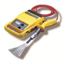
Porosity detector is a small and light weight unit with battery pack and features: digital display of applied voltage, constant test current, fully adjustable voltage and sensitivity controls. It can be used in most applications including pipeline, steel structures and tank work.
