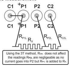
For measuring low resistance, this measuring method can be utilized C1 and P1 terminals are shorted at the tester.
