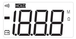
The HOLD Sign indicator comes on when the readings are held.
