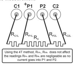
For measuring low to very low resistance (contact resistance), this is the preferred measuring method because the resistance of the test leads does not have an effect (negligeable) on the measuring results.
