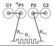
Using the 2T method, the resistance of the test leads are added to the readings. This is not recommended for low resistance and long leads.
